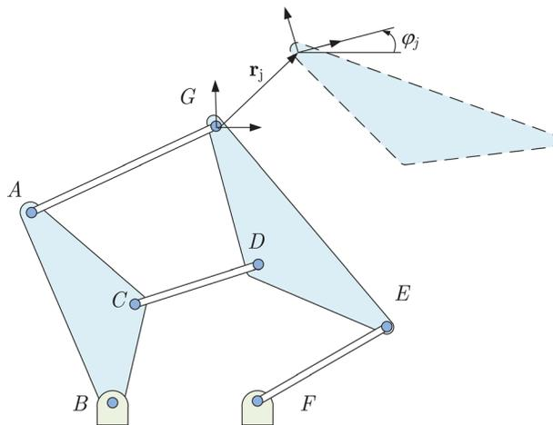
Fig. 4 The Stephenson-II linkage, where dyads  $AB$ ,  $CD$ , and  $EF$  are to be synthesized
