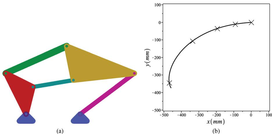
**Fig. 6 A Stephenson-II linkage synthesized: (a) CAD model and (b) a piece of coupler curve and points of visit**
