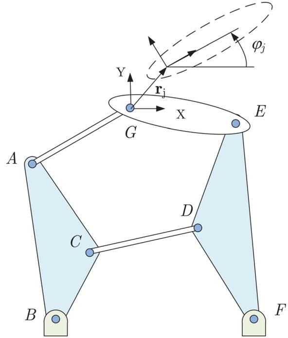
**Fig. 5 The Stephenson-I linkage, where dyads  $AB$ ,  $CD$ , and  $EF$  are to be synthesized**
