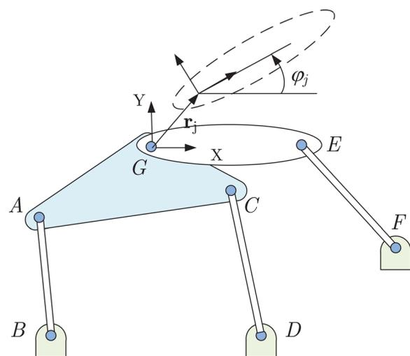
**Fig. 1** A Stephenson-III linkage. Three dyads, namely, dyads  $AB$ ,  $CD$ , and  $EF$  are to be synthesized.
