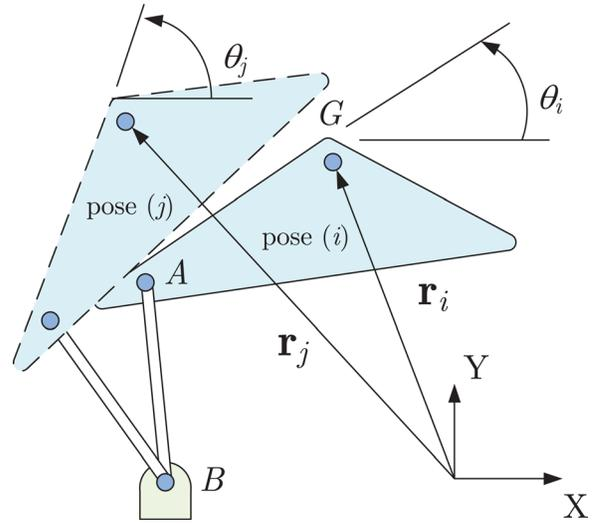
Fig. 3 Two separated poses of link *AG*
