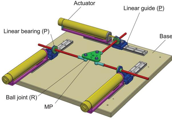
Fig. 1 CAD model of a 3-PPR PPM
