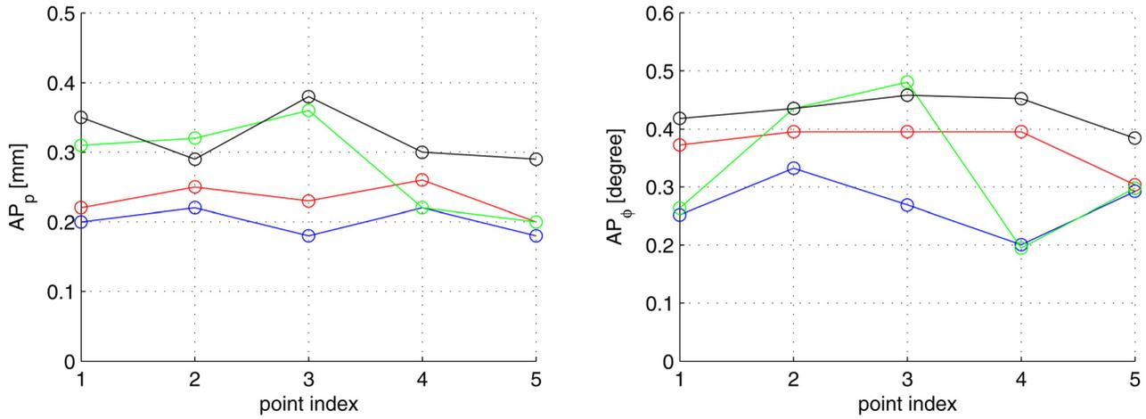
Fig. 14 Position and orientation accuracies at five poses
