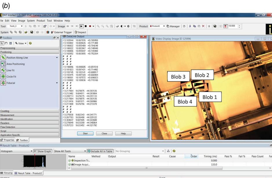
Fig. 6 A vision-based system for the moving platform pose measurement: (a) experimental setup and (b) measurement interface
