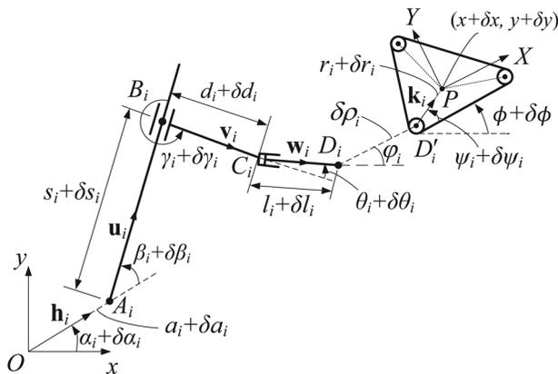
Fig. 4 Parameterization of the  $i$ th leg
