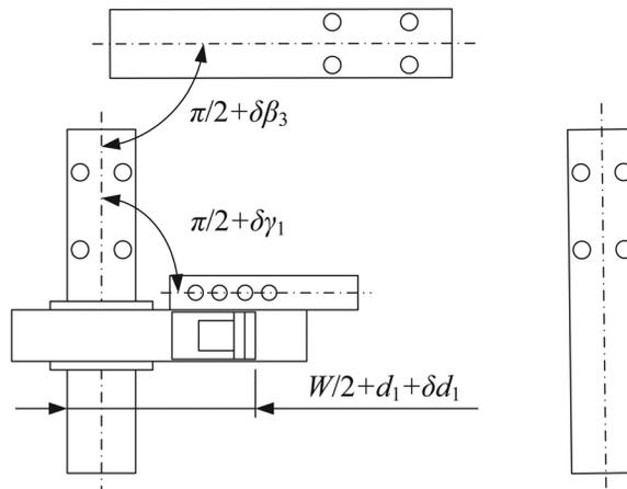
Fig. 7 Measurement of the assembly errors
