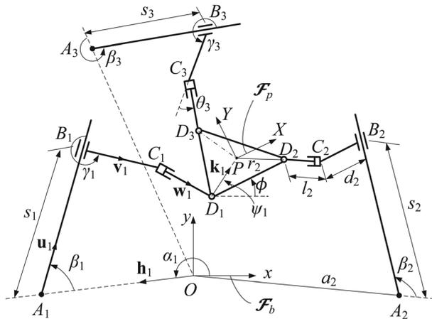
Fig. 2 Parameterization of the 3-PPR PPM
