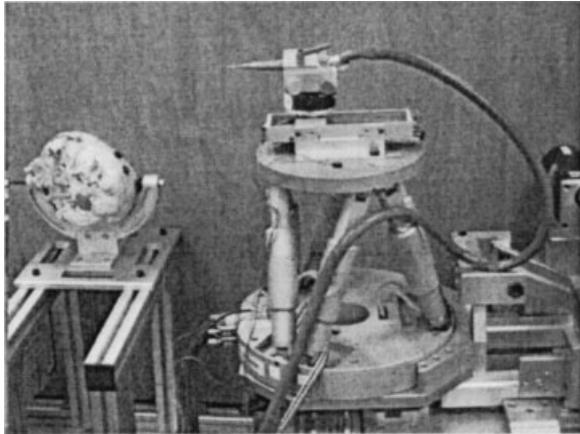
Figure 1. NEUROBOT, a medical parallel manipulator developed for neuro surgeries.
